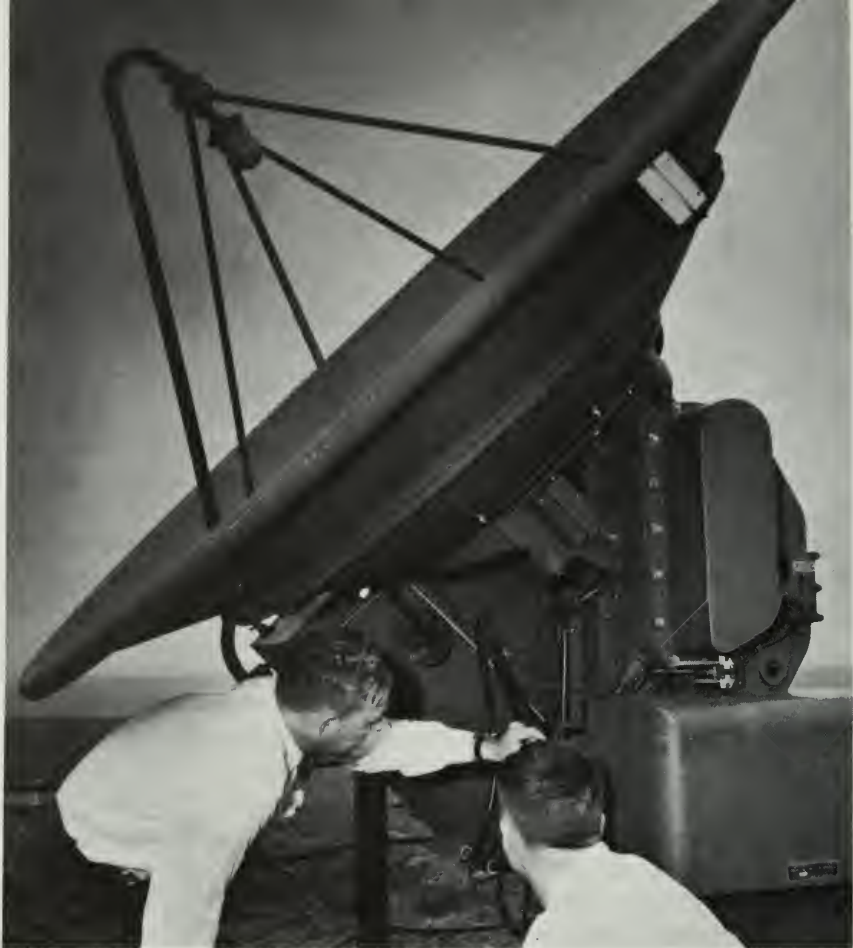
One of the radar antennae used in weather detection by the United States Weather Bureau, the Department of Commerce.
